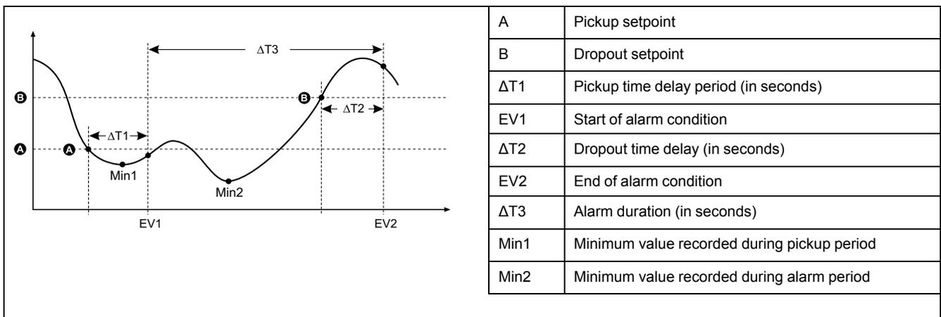
The meter records the date and time when the alarm event starts (EV1) and when it ends (EV2). The meter also performs any task assigned to the event, such as operating a digital output. The meter also records minimum values (Min1, Min2) before, during or after the alarm period.
